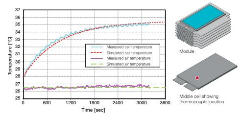
Figure 1. Good correlation of an indirect air-cool module under continuous discharge-charge condition.
