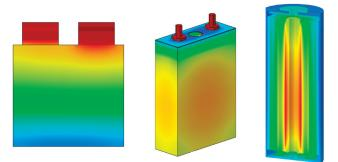
Electro-thermal model of cells of different geometries.
