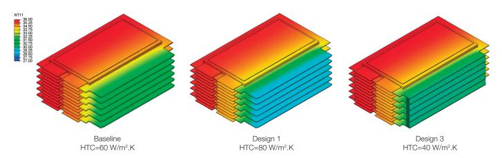
Figure 2. Abaqus FEA models of stabilized cell temperatures for three module designs with similar steady state temperatures. Compared with the baseline, Designs 1 and 3 are smaller. However Design 1 requires higher air flow.
